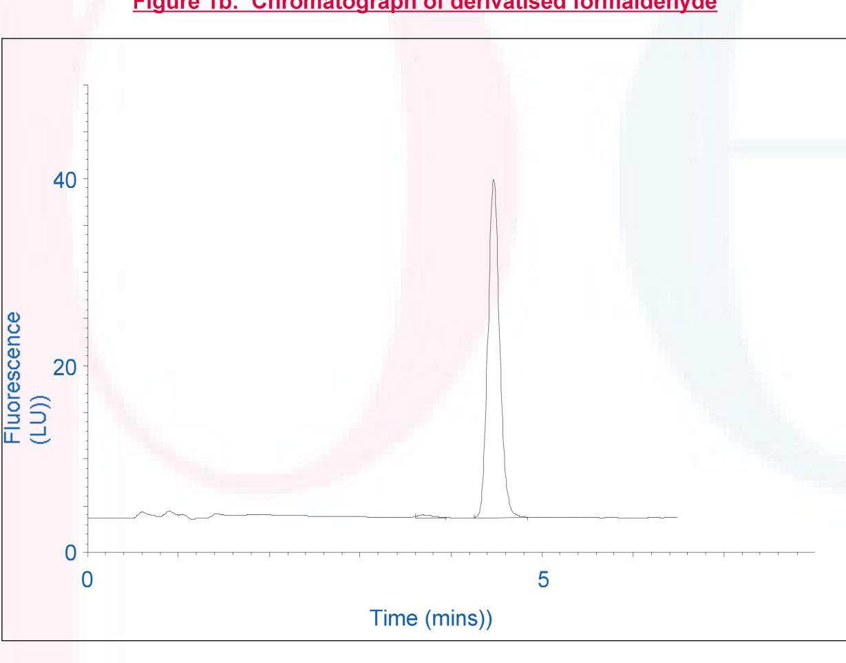
A sample of 10 μM formaldehyde in 100 mM potassium phosphated buffer, pH 7.4, 5 mM magnesium chloride (1 mL) was prepared, then 500 μL 20% trichloroacetic acid added. Following centrifugation 1 mL supernatant was incubated with Nash Reagent as described in Materials and Methods prior to injection of 50 μL onto the
