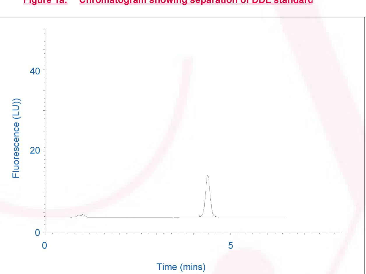
A sample of 2  $\mu$ M DDL (in ethanol) in 100 mM potassium phosphate buffer, pH 7.4, 5mM magnesium chloride (1 mL) was prepared, then 500  $\mu$ L ethanol and 20  $\mu$ L 6M HCl was added. 50  $\mu$ L was injected onto the HPLC using the conditions as described in materials and methods.
