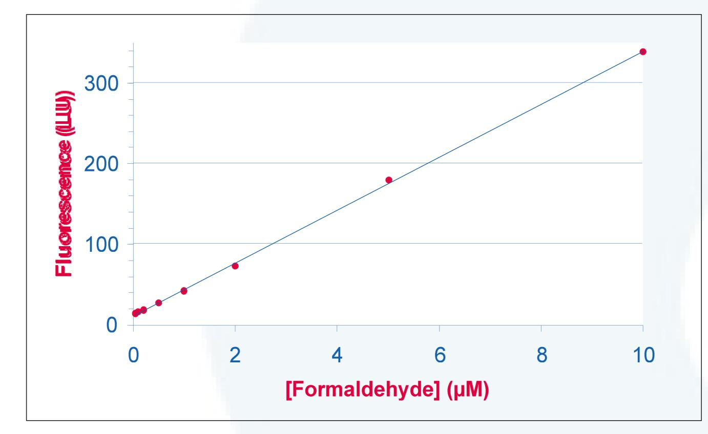
Formaldehyde standards in 100 mM potassium phosphate buffer, pH 7.4, 5 mM magnesium chloride, 1% ethanol, 40 pmol P450/mL (1 mL) were prepared, then 1 mL ethanol was added. Following centrifugation, 1 mL supernatant was incubated with Nash Reagent prior to separation by HPLC as described in Materials and Methods.
